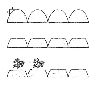
Beds are formed and **Avalaire Flumi 51 WDG** is applied with a burndown herbicide. A minimum of 2 months after **Avalaire Flumi 51 WDG** application, the tops of the beds are removed and the soil from the tops of the beds is placed in the area between the beds. Crops are transplanted into beds.
