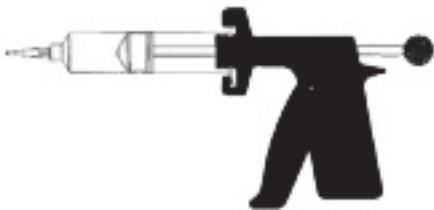
Schematic representation of the Mylva Imidacloprid Ant Bait applicator gun
