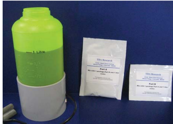
Figure 6: Salts and surfactants ready to be poured into the 1 liter of water in the bottle
