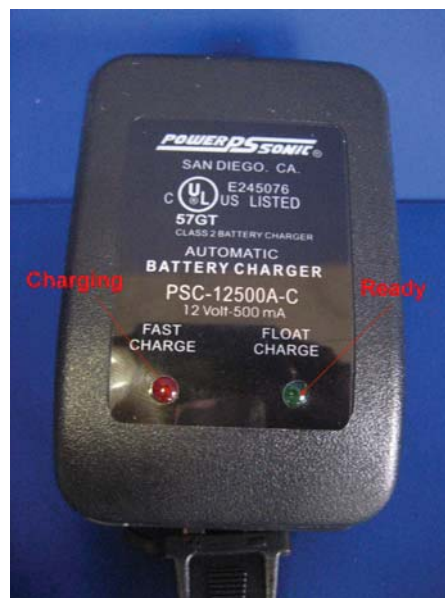
Figure 10: HDA Battery Charger
