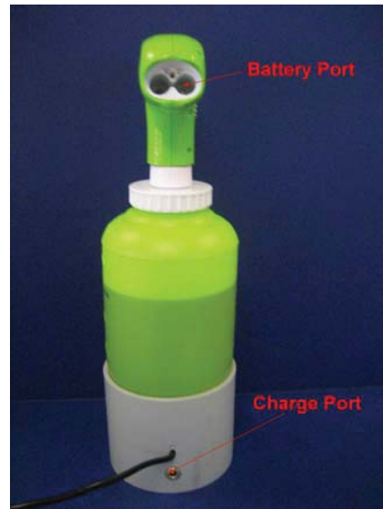
Figure 7: Spray head replaced onto the bottle displaying alignment of the spray head and charge port
