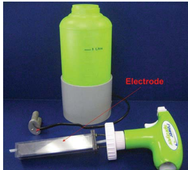
Figure 4: Spray head removed from bottle displaying electrode
