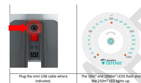
The device will not diffuse when in USB mode. To exit USB mode, unplug the cable
