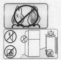
{graphic size 2.25 cm x 3.5 cm minimum} Turn off ALL ignition sources such as pilot lights (shut off gas valves), other open flames or running electrical appliances that cycle off and on (i.e., refrigerators, thermostats, etc). Call your gas utility or management company if you need assistance.
