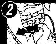
2 Slide white strip on cap. Then grab "T-handle" and pull all the way up. JUST PULL UP - NO NEED TO PUMP.
