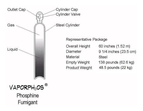
The product flows to the blending equipment through the cylinder outlet valve. As gas is withdrawn from the cylinder, some of the product vaporizes to fill the remaining space in the cylinder. Through this
