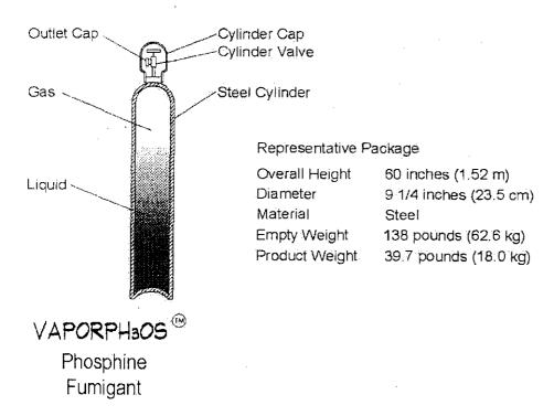
withdrawn from the cylinder, some of the product vaporizes to fill the remaining space in the cylinder. Through this vaporization, the cylinder pressure is maintained.
