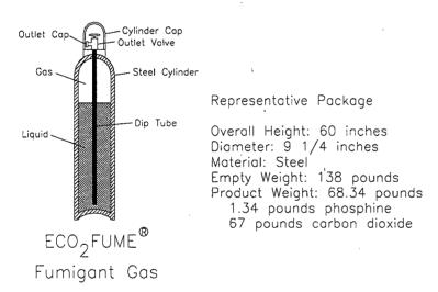
As liquid is withdrawn from the cylinder, some of the product vaporizes to fill the remaining space in the cylinder. Through this vaporization, the cylinder pressure is maintained.
