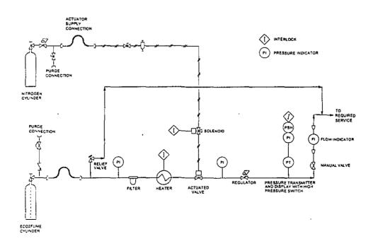
Diagram of a Representative Type of ECO<sub>2</sub>FUME® Dispensing Equipment
