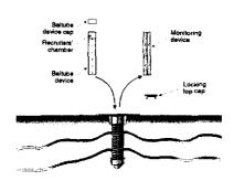
**1b.** Remove termites from the monitoring device into the collecting pan and introduce them into the top of the Baitube.
