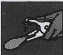
Figure 2. Slide male button on pin. Align tip of male button with female portion of tag. Tag and button are now ready for application.
