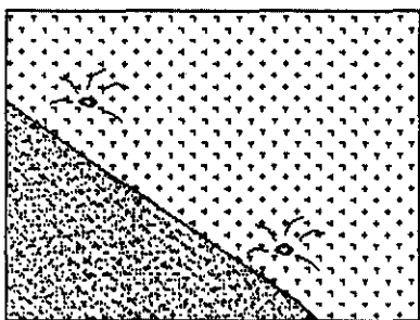
D. Secure fabric edges by cutting a shallow trench (approx. 1") & 'toeing in' edge of Biobarrier into trench. Peg fabric edge in trench every 4'
