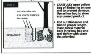
Beginning at one end of the trench, hold product in place at finished grade level on the side of the trench adjacent to the hardscape (opposite root source) and stake in position using pins provided. Use Caution when handling installation pins - they are sharp.
