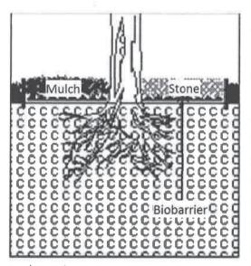
(provided in package). "Toe-in" or press outside edges of Biobarrier<sup>®</sup> down into trench. Insert landscape pins at 1' intervals around perimeter of skirt.
