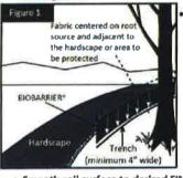
Cut all roots back flush to trench walls on both sides of trench. For some species, it may be neces-sary to spray the cut end of the severed root on the side opposite tree to prevent root regrowth under the hardscape. If this is necessary, use a systematic herbicide and be extremely careful to avoid contact with roots on the opposite side of the trench.
