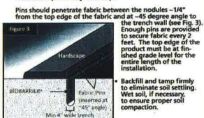
Backfill and tamp firmly to eliminate soil settling. Wet soil, if necessary, to ensure proper soil compaction.
