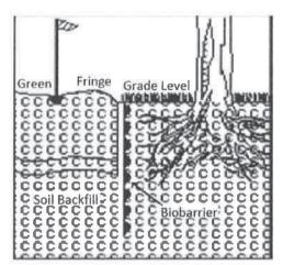
Dig a clean trench (extending to depth below existing roots) where Biobarrier<sup>®</sup> is to be installed. Remove roots on both sides of trench. Place top edge of Biobarrier<sup>®</sup> at finished grade level, securing with installation strips and/or pins provided, insuring that product hangs straight and taut, with no slumping or gaping. Backfill, compacting soil firmly. Biobarrier<sup>®</sup> may need to go deeper under these ideal growing conditions.
