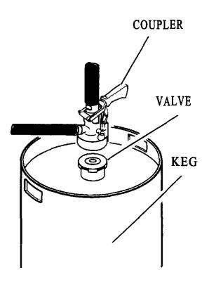
**IMPORTANT!** Attach a hose or pump to the coupler before engaging coupler. This will prevent the user from being splashed in the event that pressure build-up in the keg forces liquid up through the coupler.
