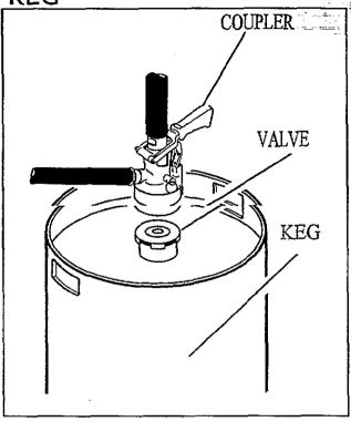
IMPORTANT! Attach a hose or pump to the coupler before engaging coupler. This will prevent the user from being splashed in the event that pressure build-up in the keg forces liquid up through the coupler.
