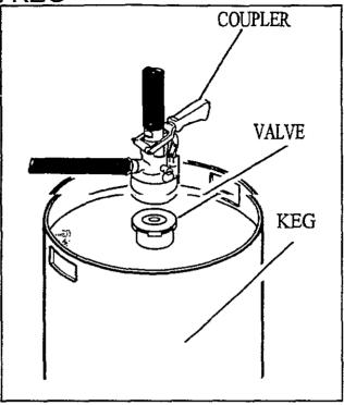
IMPORTANT! Attach a hose or pump to the coupler before engaging coupler. This will prevent the user from being splashed in the event that pressure build-up in the keg forces liquid up through the coupler.
