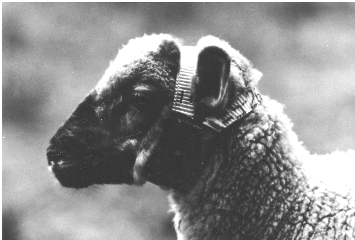
Photo 6. Elastic-strap LP Collar on a 50-pound lamb. In field tests on Angora goats the rate of collar puncture by attacking coyotes was lower for elastic-strap than for Velcro-strap collars.
