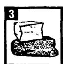
OPEN BAG AS FOLLOWS: Carefully open this beg at the perforation and immediately drop the inner bag into the mix tank. Do not open or handle the inner bag - Moisture will cause breakage.
