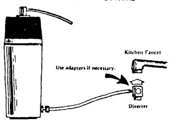
Unscrew aerator off kitchen faucet, Screw on diverter (use adapter if necessary). Push diverter valve one way for filtered water and the other for tap water through faucet.
