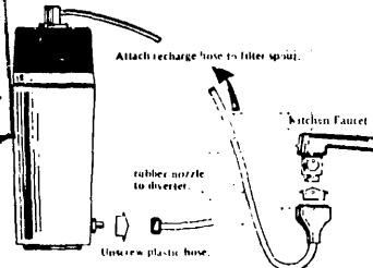
Every four to six weeks attach recharge hose to lifter spour, unscrew plastic hose from lower unit litting, place universal fitting over faucet diverter and backwash for 10 to 15 minutes. Then, reconnect as before. Depending on water quality backwash may only be necessary every three to four months.
