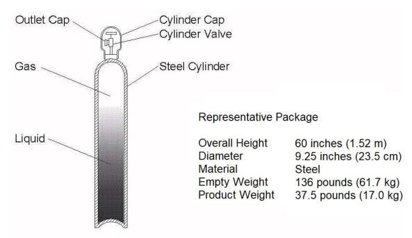
The product flows to the blending equipment through the cylinder outlet valve. As gas is withdrawn from the cylinder, some of the product vaporizes to fill the remaining space in the cylinder. Through this vaporization, the cylinder pressure is maintained.
