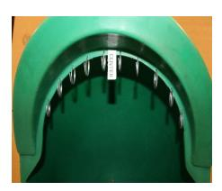
**Step 1** - Using a 1/8" bit, drill 10 holes for kick out rings in the edge of the upper arch of the mineral feeder opening. Make a mark at the center edge of the top arch of the opening (12 O'clock). Starting 1 inch from the right of the center mark drill 5 holes 1- 3/4 inches apart in the edge of the arch opening. Repeat 5 holes for the left hand side of the center mark. The holes need to be approximately 1/8 to 1/4 of an inch from the edge of the feeder opening.
