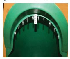
**Step 1** - Using a 1/8" bit, drill 10 holes for kick out rings in the edge of the upper arch of the mineral feeder opening. Make a mark at the center edge of the top arch of the opening (12 O'clock). Starting 1 inch from the right of the center mark drill 5 holes 1- 3/4 inches apart in the edge of the arch opening. Repeat 5 holes for the left hand side of the center mark. The holes need to be approximately 1/8 to 1/4 of an inch from the edge of the feeder opening.
