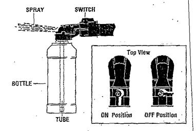
To Start Flow of Insecticide: Turn on water supply. Line up switch on top of sprayer directly with hose. Spray evenly and completely over lawns and other infested areas, giving special attention to areas frequented by pets. Hold about three feel above surface, moving at a steady pace to insure consistent, thorough coverage.
