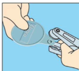
Figure 2. Slide tag under the clip of the pliers by depressing the lever.
