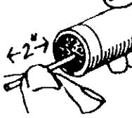
**3. Light fuse and insert cartridge into runway opening. Minimum fuse burning time 5 seconds**
