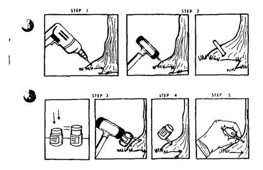
Measure DBH (Diameter Breast High) in inches and divide by two to determine the number of capsules to use. Transfer placement to root collar (about 4 inches above ground level) on the stimulated root flares or high points. (See back of Page)
