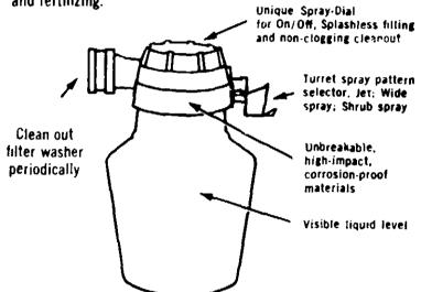
For proper operation of sprayer, be sure arrow on handle is directly in line with spray position selected on dial. This will click into position when properly set.
