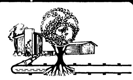
Chief cause of sluggish sewers, cesspool and septic tank drain lines is stoppage by tree and shrub roots in pipes.
