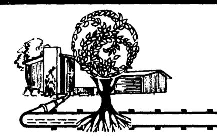
Chief cause of sluggish sewers, cesspool and septic tank drain lines is stoppage by tree and shrub roots in pipes.
