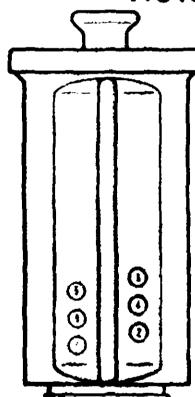
STEP 1. Remove red plug from hole indicated for gallonage nearest your pool size.
