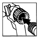
1. Attached garden hose to spray nozzle and turn on water supply.
