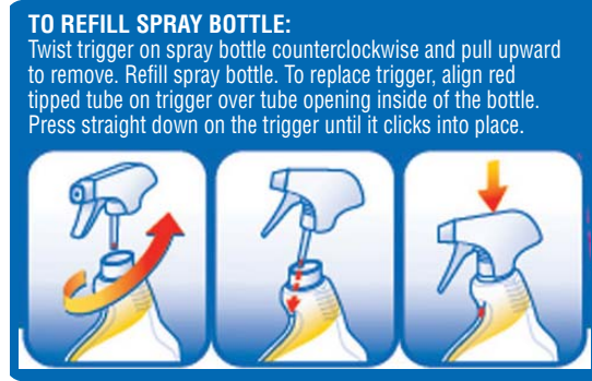
Twist off, Refill Align Tip to Tube Push, Snap to Close
