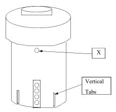
5. To make the initial height setting of the cartridge in the feeder, select the number on the graduated scale on the side of the cartridge according to the gallon capacity of your pool as determined by the chart below:
