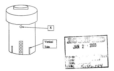
5. To make the initial height setting of the cartridge in the feeder, select the number on the graduated scale on the side of the cartridge according to the gallon capacity of your pool as determined by the chart below:
