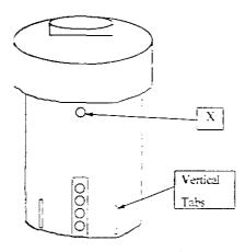
5. To make the initial height setting of the cartridge in the feeder, select the number on the graduated scale on the side of the cartridge according to the gallon capacity of your pool as determined by the chart below:
