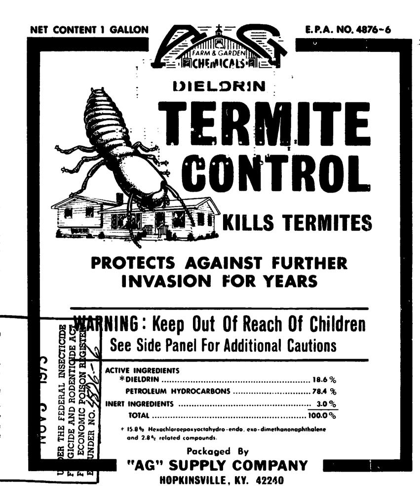
The basic principal of termite control is to place an impregnable barrier between the termites and the building to be protected. This barrier must be complete, for termites are quick to seek out unprotected way to a food supply. A chemical barrier of Dieldrin is most satisfactory because termites cannot live in or pass through Dieldrin-treated soil. Dieldrin persists in the soil for years-giving long protection against reinfestation.
