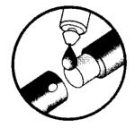
(Assembly Tip: To make assembly easier, add a small drop of liquid soap at the tip of the connector, then insert and twist! To improve grip during assembly, use rubber gloves.)
