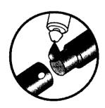
(Assembly Tip: To make assembly easier, add a small drop of liquid soap at the tip of the connector, then insert and twist! To improve grip during assembly, use rubber gloves.)
