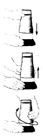
(Pictures to go near "Warning: top surface of lamp is very hot. Do not touch top surface")
