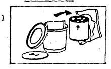
Tear off the plastic outer seal covering: the: fogger. Remove the yellow cardboard cover and discard. Take out the inner container and remove its portective foil pouch. Use care not to tear or destroy the red seal covering the metal can.
