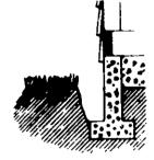
Remove soil from around building leaving a trench 12 inches deep. Soak soil with solution using 1 gal-Ion per 2 cubic feet or 1 gallon per 2 lineal feet of trench. For buildings with deep foundations, a 30 inch deep trench is recommended and solution applied at rate of 1 gallon per lineal foot. Do not spray solution on any part of plants. Grass. plants, and other shrubbery within three feet of trench should be removed or protected. Trench should not be dug below top of footing.
