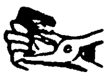
2. Place tag under retainer plate. Raised square must be facing up. Tag and rivet are now ready for application.
