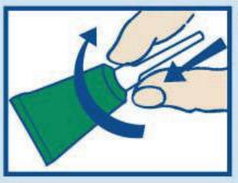
2 Twist dispensing tip clockwise about ½ turn while pushing down to break the tube's seal. Do not remove the dispensing tip.
