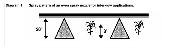
The broadcast dosage rates must be adjusted for this "inter-row" application. Specifically, multiply the broadcast dosage rate times the fraction of the row width covered by the spray pattern. Or, use the formulas below to compute the proper dosage rate and spray volumes for this inter-row method of application.
