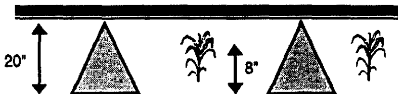
Diagram 1: Spray pattern of an even spray nozzle for inter-row applications.
