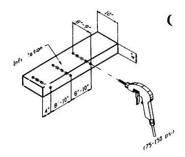
FIGURE 2: Alternative pressure treatment of a 4"x10" structural beam.
