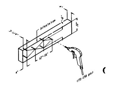
FIGURE 1: Drill and pressure injection of a 4"x10" structural beam with 10% TIM-BOR solution.
