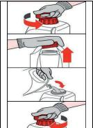
Remove the pump handle on the Quick Pump/Applicator Name by twisting it counterclockwise. [Illustration]
