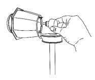
8. Replace [re-attach] [Fixture] [Device] [Unit] cover.
