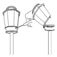
6. Ensuring that the locking adaptor cap is secured to the [Repellent Bottle] [Repellent Cartridge] [Repellent Refill], carefully insert MGK FORMULA 3163 [bottle name] [Repellent Bottle] [Repellent Cartridge] [Repellent Refill] into fixture so that top of wick fits into Vaporizer [Liquid] [Repellent] [Emanator] and rotate about 30 degrees to secure to fixture [device] [unit].
