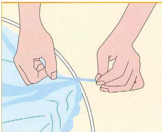
Unfold net and turn inside out to attach hoop to net. To set, tie all (six) strings securely to the ring.
