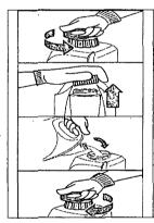
Remove the pump handle on the Quick Pump/Applicator Name by twisting it counterclockwise. [Illustration]
